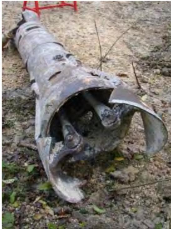
**Figure 52. Benne de havage**
